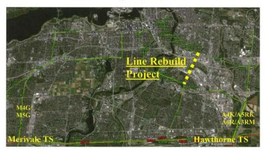
With forecasted load growth in the downtown area, the main section of A4K, from Hawthorne TS to Blackburn JCT, will exceed planning criteria starting 2017. Upon the contingency of losing the companion circuit A5RK, A4K will experience thermal overload.
