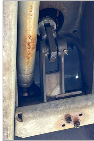
(b) Switching equipment lubrication leaks
