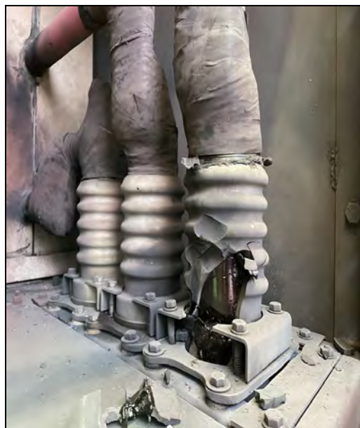
(f) Pothead failure connected to station bus
