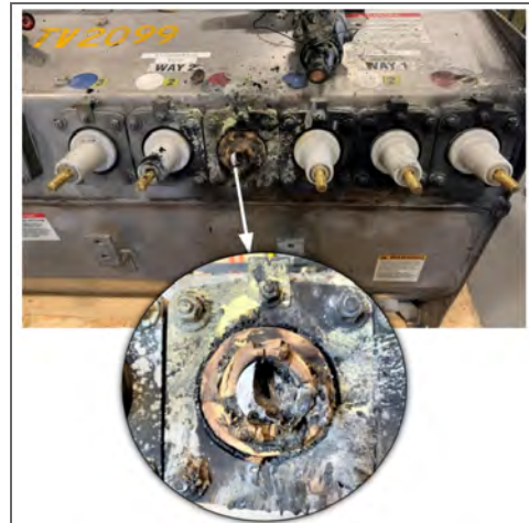
Figure 57 - Vault Switchgear Failure
