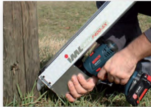
FIGURE 6.3 - IML RESISTOGRAPH DRILL
