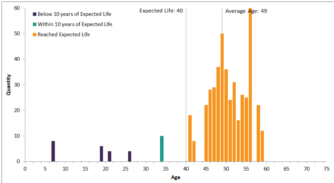
Figure 6.18 – Station Electromechanical Relay Demographics
