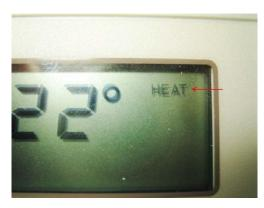
**Step 2**. The display will change to "**HEAT**". Set the temperature to your desired temperature (higher than the current room temperature). You will hear a faint "click" and the heat will come on.
