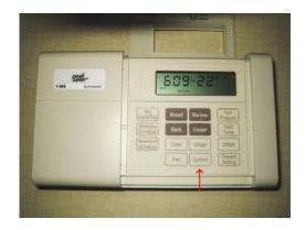
**Step 1**. Open the door and press the "**SYSTEM**" button until the word "**HEAT**" is in the upper right corner of the display.
