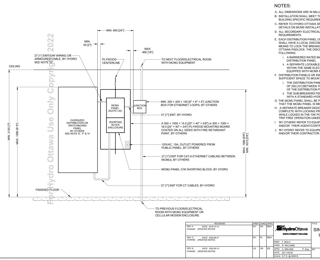
G:\4.2.3 TECH STD & MAT\01\_STDS\01 HOL\M-METERING\C-CONSTRUCTION\MCS0059 R6 SINGLE MULTI-CUSTOMER METERING UNIT WITHOUT COMMUNICATION EQUIPMENT.DWG
