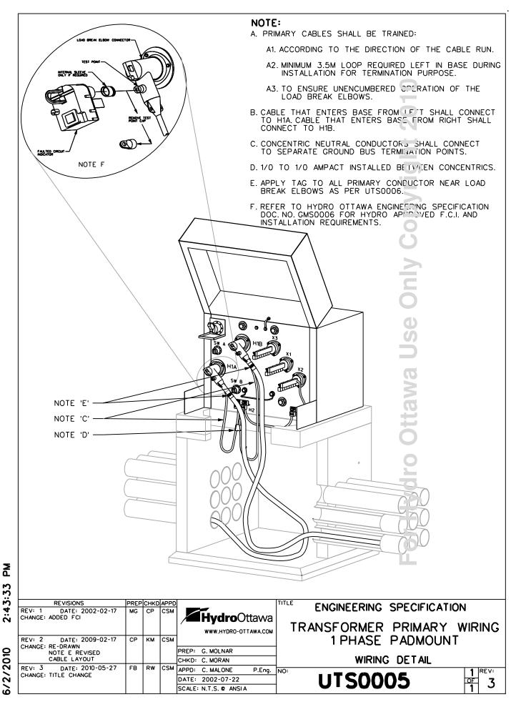
K:\STANDARDS\U-Underground\T-transformer\UTS0005 R3 Transformer Primary Wiring 1PH Padmount.d
